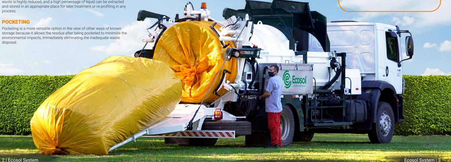
The Ecosol system comprises an Ecotruck and some auxiliary equipment that allow the moving and optimization of the pocketing process.
